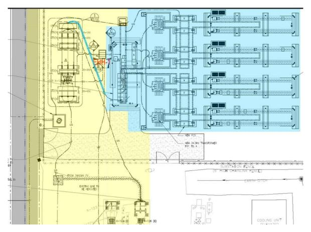
The communication network infrastructure at the Agana site will be operated and maintained by GPA within the yellow areas shown in the drawing below and the network infrastructure at the Agana site will be operated and maintained by Contractor within the blue areas shown in the drawing below
