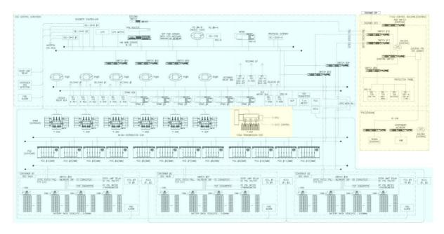
The communication network infrastructure at the Talofofo site will be operated and maintained by GPA within the yellow areas shown in the drawing below and the network infrastructure at the Talofofo site will be operated and maintained by Contractor within the blue areas shown in the drawing below
